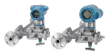
Rosemount 3051CFP Integral Orifice Flow Meters enable highly accurate flow measurement in small line sizes. Integral Orifice Flow Meters use precision honed pipe section for increased accuracy and self-centering plate design to prevent alignment errors that magnify measurement inaccuracies in small line sizes.
