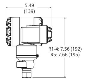
Figure 11: Rosemount 3051T In-Line Range 6
