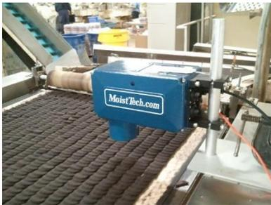
Measuring moisture content throughout the process also provides snack food manufacturers cost savings in energy and fuel costs, as well as having less product waste. With continuous NIR online moisture testing, manufacturers can monitor moisture levels which they in-turn, can precisely control ovens and fryers to optimize the production process with minimum energy requirements as well as preventing over cooking.
