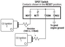
VS2EX Typical Wiring Diagram for Single or Dual CD Ignitions
